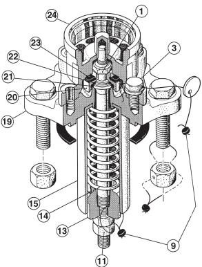
Disassembly of the Top Guide and O-ring Retainer
